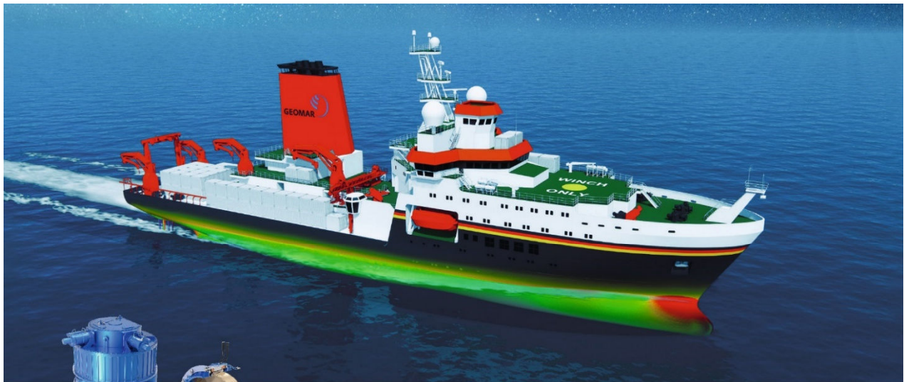
The new German research vessel METEOR IV propelled by 2 x eVSP 32X8/285 and VIT 2000-1650H
