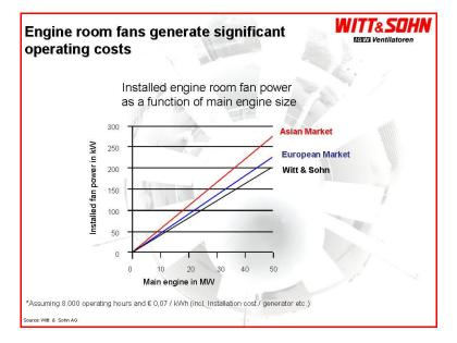
Differences of 20% in the efficiency factor are normal. Comparing the relatively low efficiency factors of 70-80% for poorly-produced Asian electrical motors to the 90-95% efficiency factors in Europe shows dramatic differences.
