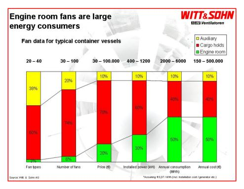
Aside from the main engine, the engine room fans are the most costly machinery, in energy terms, on board a ship.
